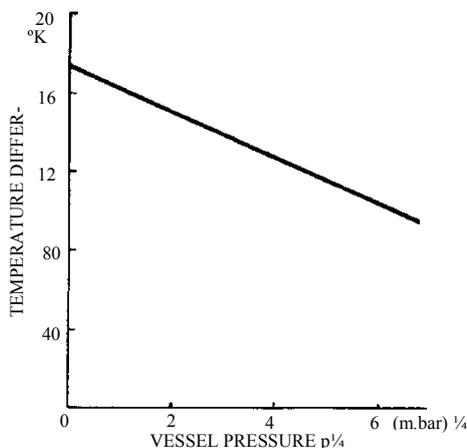
FIG. 2 Temperature Difference v Vessel Pressure
