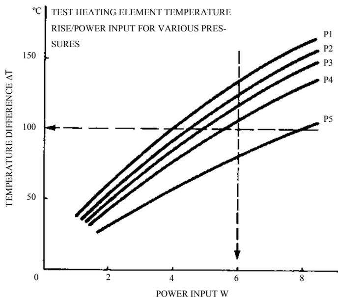
FIG. 1 Temperature Difference v Power Input
