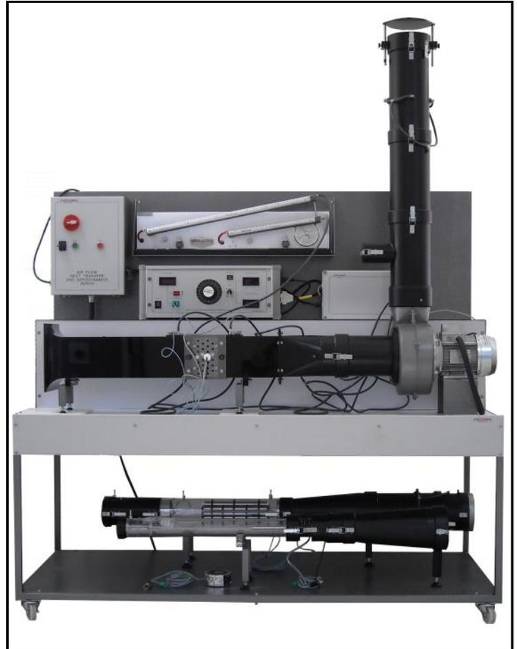
The relationship between Nusselt, Prandtl and Reynold's numbers can be investigated by varying the air flow rate, the electrical power to the model and hence the surface temperature. The effect of the change of air flow rate on the pressure drop over the test models can also be investigated. The velocity of the air flow in the test section is determined by means of a pitot static tube.
